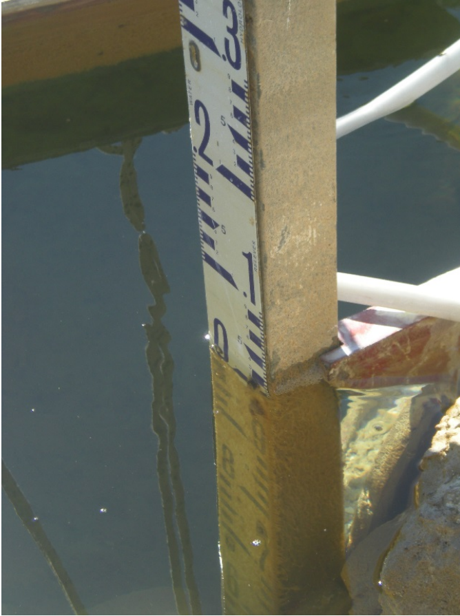
Photograph 14: Main Pond Water Level at Culvert Intake to Settling Pond (201.03 m). 27 July 2017
